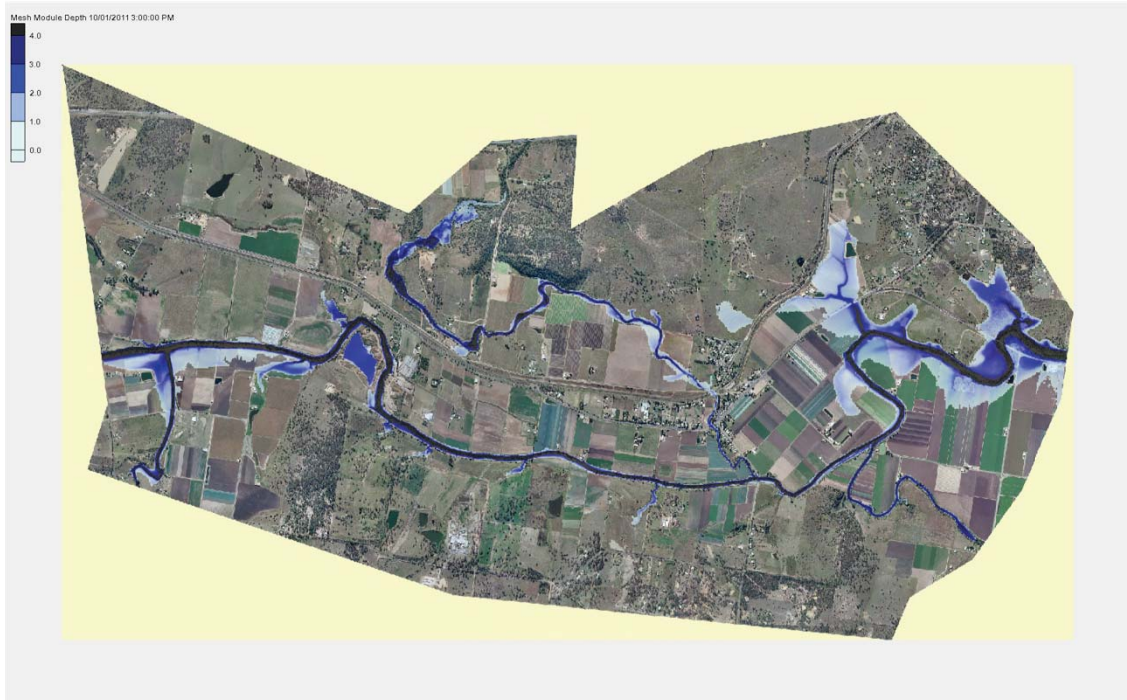
Figure B.16 – Initial Flood Flow Inundation using LVRC ULG Downstream Rating
