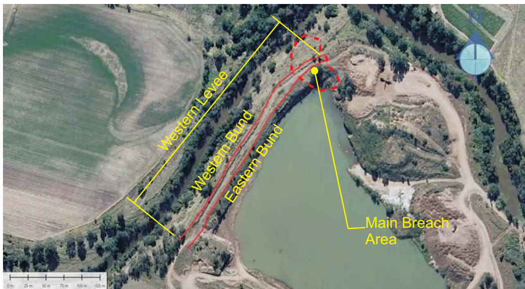
Figure 8.15 – Alignment of Pre Flood Quarry Bunds and Location of Main Breach
