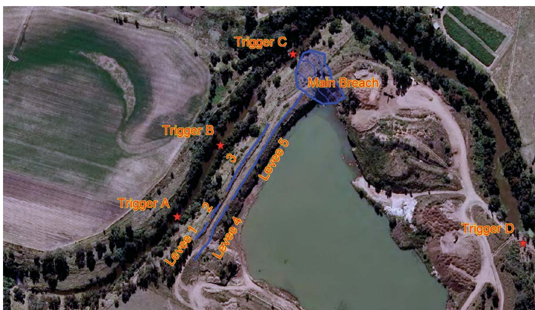
Figure 10.9 – Quarry Failure Trigger Level Locations
